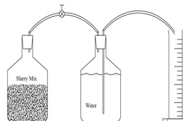
**Figure 2:** Schematic of the anaerobic digestion experiments.
