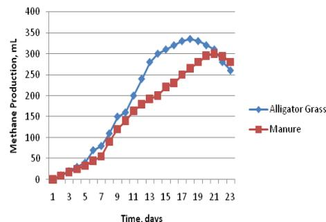
**Figure 3:** Plots of biogas production with time during anaerobic digestion experiments.
