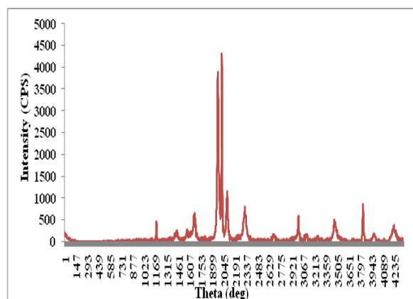
**Figure 1:** XRD patterns of Nano-ZnO-Magnetite.
