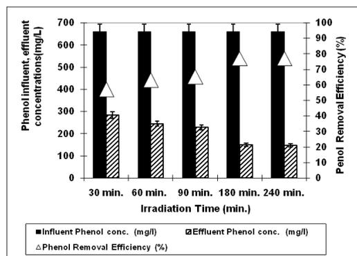
Figure 3: The effect of Irradiation time on phenol yield (Influent Conc.: 660 mg/L, T: ±20 °C, pH: 4.00, Nano-ZnO-Magnetite concentration: 3g/L, UV power: 300 W).
