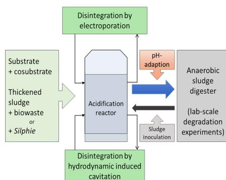
Figure 1: Experimental setup of semi-scale acidification reactor.
