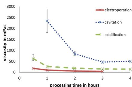
Figure 3: Reduction of viscosity of thickened sludge by impact of electroporation and cavitation.
