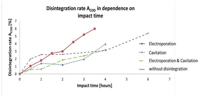
Figure 2: Disintegration rates A<sub>COD</sub> of thickened sludge by acidification and disintegration.
