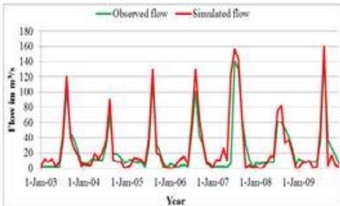
Figure 7: Observed and simulated flow hydrographs during calibration period.
