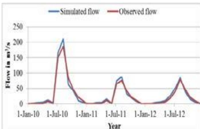
Figure 9: Observed and simulated hydrographs during validation period.
