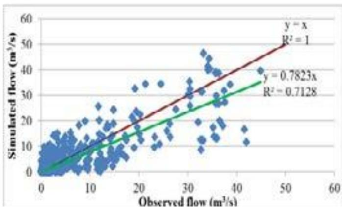
Figure 8: Scatter plot during calibration period in the Geba catchment.
