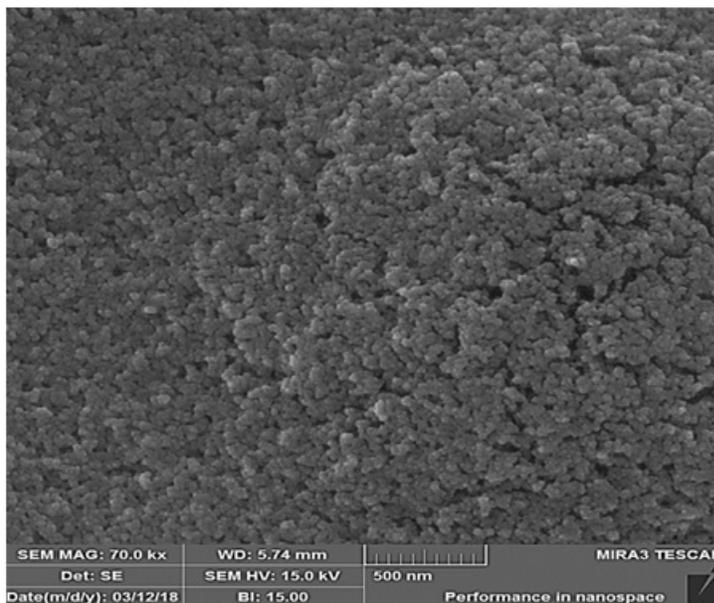
**Figure 4:** SEM image of the produced chitosan/extract nanoparticles
