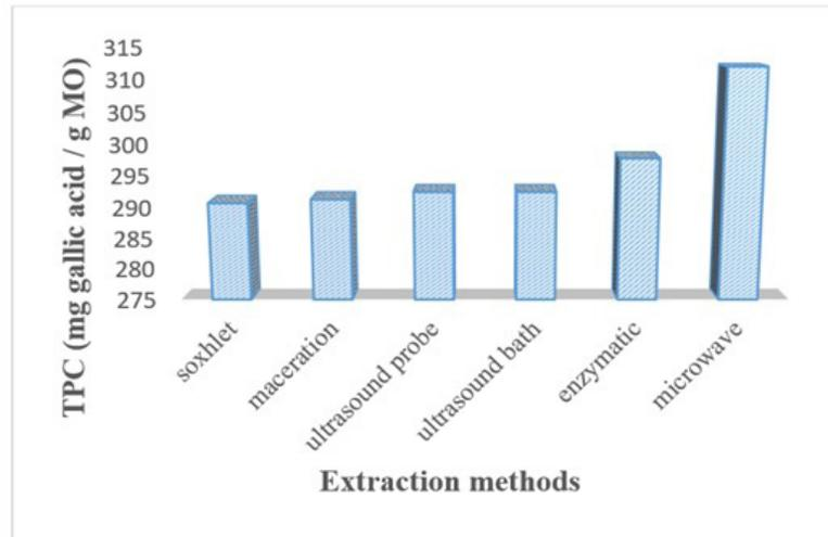
**Figure 1:** The effects of using different extraction methods on TPC (mg gallic acid/ g MO)
